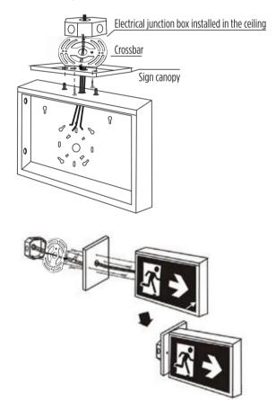
4. Reference step 4-7 in wall mounting above for ceiling or end mounting.
