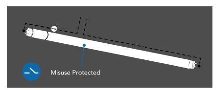
Misuse - Protected function if forgot to by-pass the ballast, the lamp won't work, no risk of fire or cap melting.
