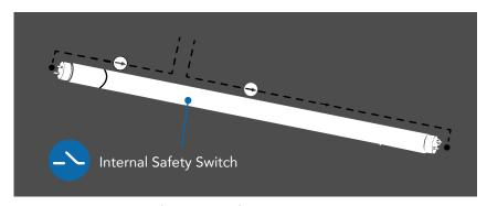
Internal Safety Switch for installation protection. (No current will flow until pins on both ends are engaged)
