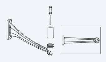
Step 3: Align the screw holes on the sleeve with those on the wall bracket one by one, then tighten the screws onto the sleeve.
