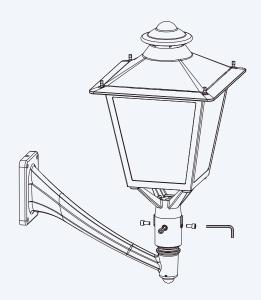
Step 5: Insert the mounting bracket into the sleeve, and tighten the four screws with a hex key wrench.
