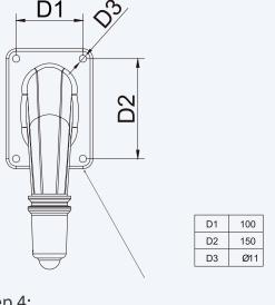
Step 4: Drill holes in the wall, then install 12mm-long M8 expansion bolts.
