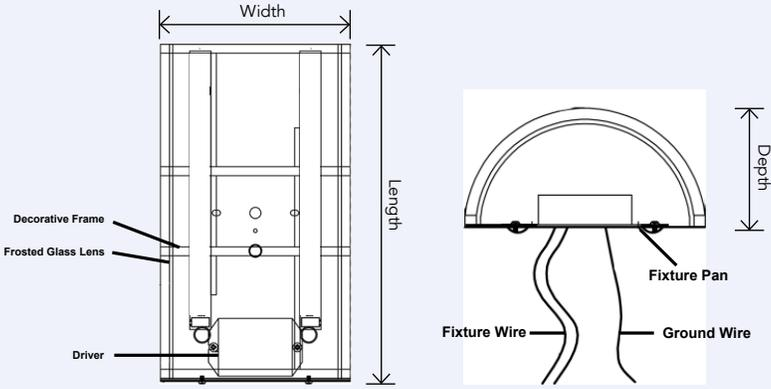
The technical drawing consists of two views. The left view is a front elevation showing the 'Decorative Frame', 'Frosted Glass Lens', and 'Driver' components. It includes dimension lines for 'Width' and 'Length'. The right view is a side elevation showing the 'Depth' of the fixture, the 'Fixture Pan', and the 'Fixture Wire' and 'Ground Wire' connections.
